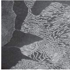
Scanning electron micrograph showing the microstructure of a steel that contains 0.44 wt% C. The large dark areas are proeutectoid ferrite. Regions having the alternating light and dark lamellar structure are pearlite; the dark and light layers in the pearlite correspond, respectively, to ferrite and cementite phases. 700 \times . (Micrograph courtesy of Republic Steel Corporation.)
