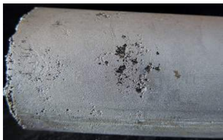
Figure 17.17 Pitting of a 316L stainless steel pipe surface by a phosphate solution. (Photograph courtesy of Rick Adler/Adler Engineering LLC of Wyoming USA)
