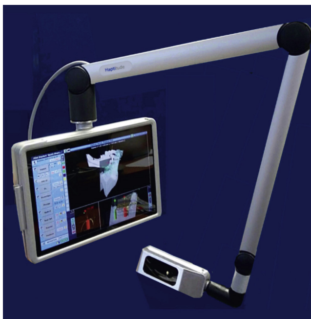
• Fig. 46.3 Dental Implant Real-time Navigation System. This figure (Open Pilot System, Stereovision Haptitude) shows a device with infrared stereovision cameras and a monitor display showing the three-dimensional ultrasonic reconstruction of a mandible with the planned implant position in a coronal and a panoramic view. (From Newman, M.G., Takei, H.H., Klokkevold, P.R., et al. (2019). Newman and Carranza's Clinical Periodontology (13th ed.). Philadelphia: Elsevier.)
