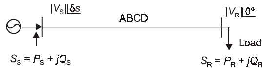
Fig. 6.7: Two bus sample power system.
