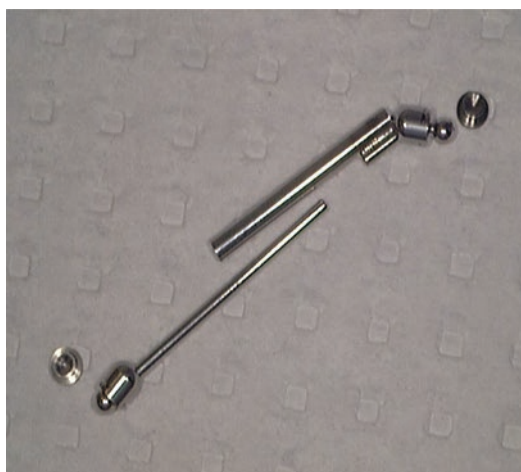
Fig. 5.6 The male and female piston configuration with the lugs that are welded to the stainless steel crowns. The ball and socket arrangement facilitates lateral movements with minimal torquing effects on the welded attachments
