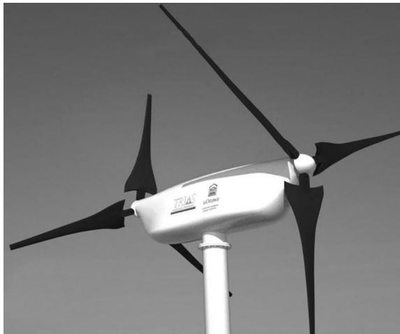
FIGURE 8.20 Example of a counter-rotating wind turbine. ( https://decoratex.biz/bsn/en/new-vetrovye-elektrostancii-dlya-doma-svoimi-rukami-opisanie-vidy-i-moshhnost.html .)
