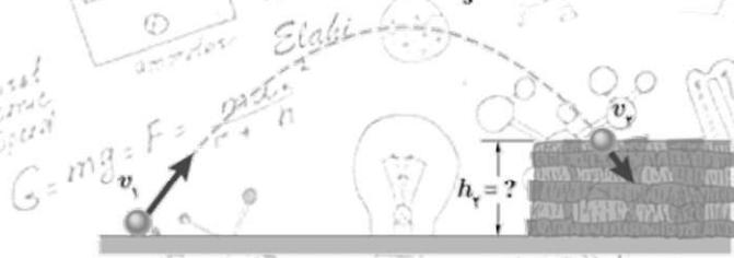
$E_1 = E_2 \rightarrow K_1 + U_1 = K_2 + U_2 \rightarrow \frac{1}{2}mv_1^2 = \frac{1}{2}mv_2^2 + mgh_2$
