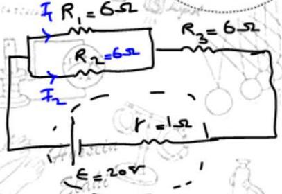
$R_{eq} = 9 \Omega \rightarrow \frac{R_1 R_2}{R_1 + R_2} + R_p = 9 \Rightarrow \frac{R_1 R_2}{R_1 + R_2} = 9 - R_p = 3$
