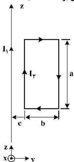
$$\bar{F} = \frac{\mu_0 I_1 I_2 ab}{4\pi b(a+b)} \bar{a}_y \quad (1)$$
