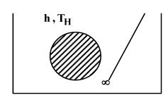
$$\frac{T - T_{H}}{T_{\circ} - T_{H}} = 1 - \frac{t}{\tau}$$
