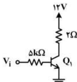
$$(V_{CESAT} = 0.2V \text{ و } V_{BE} = 0.7V, h_{fe} = 118)$$
