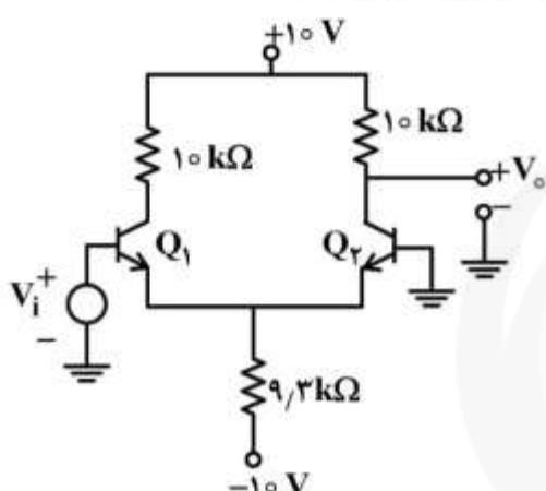
$(V_{BE} = 0.7V, \beta = 100, V_T = 25\text{ mV})$
