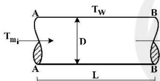
$$T_{m_0} = T_w \left[ 1 - \exp\left(\frac{-\bar{h}L}{\rho C_p D u_m}\right) \right] \quad (1)$$
