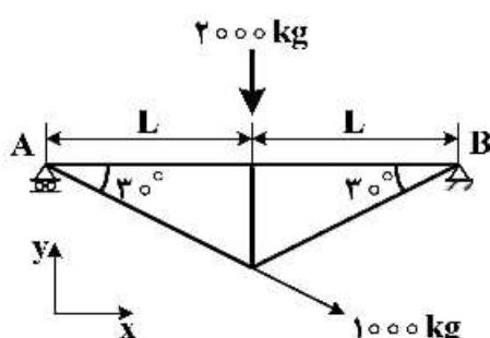
$$\begin{aligned} Ay &= 1500 & By &= 1000 \\ Ax &= 0 & Bx &= -866 \end{aligned} \quad (1)$$
