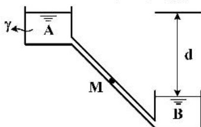
$$\begin{array}{ll} \gamma Qd & (1) \\ 4\gamma Qd & (2) \\ 2\gamma Qd & (3) \\ \frac{\gamma Qd}{2} & (4) \end{array}$$
