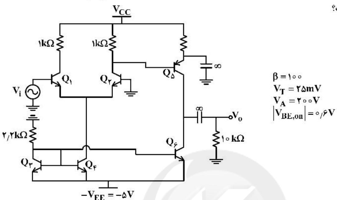
$$\begin{aligned}\beta &= 100 \\ V_T &= 25mV \\ V_A &= 200V \\ |V_{BE,ON}| &= 0.6V\end{aligned}$$
