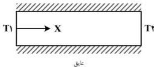
$$\frac{d^\gamma T}{dx^\gamma} + \frac{1}{b} \left( \frac{dT}{dx} \right)^\gamma + \frac{MT}{b} = 0 \quad (1)$$
