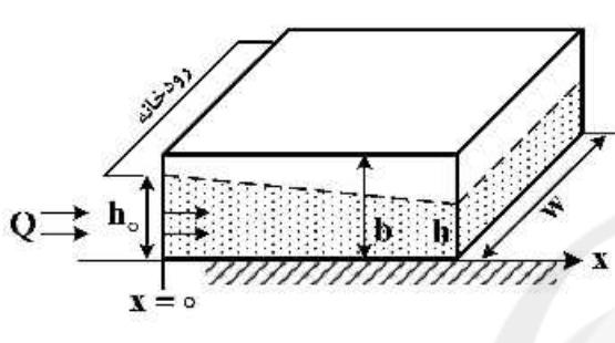
$$Q = -Kwh \frac{dh}{dx} \quad (1)$$
