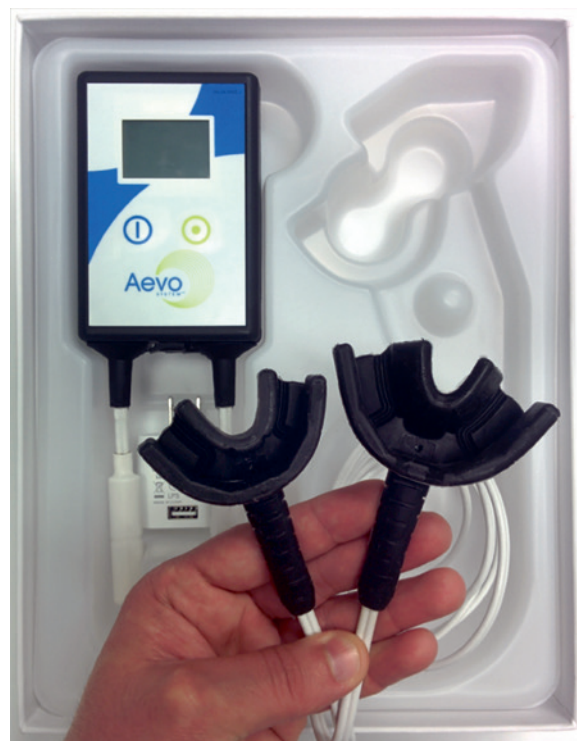
• Fig. 8.21 The Aevo device has four components: maxillary and mandibular mouthpieces with facial and lingual emitters and five treatment zones, a coupling gel for use in the mouthpieces, and a battery-powered energy source. It is used with an interface that allows selection of which treatment zones are activated and monitors patient compliance so that the doctor knows whether it is being used and how much.
