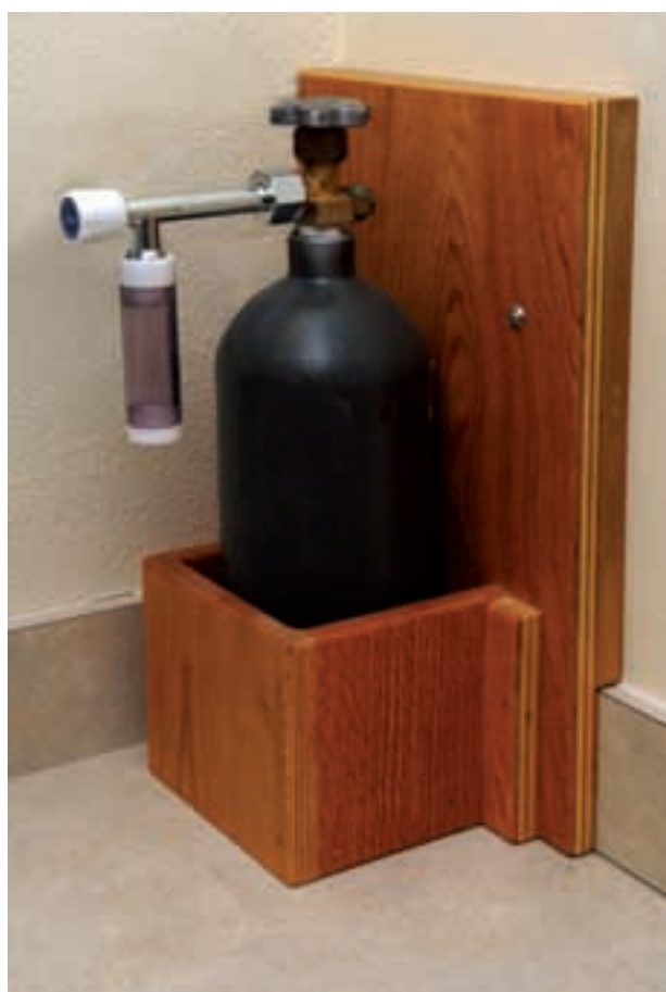
Figure 3 The CO 2 tank is stored securely in a box.
