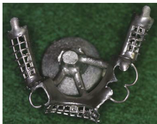
FIGURE 19-23 Mandibular cast framework with sprue intact, showing three 8-gauge sprues attached to the lingual bar. If one is concerned about completely filling distal extension base minor connectors, 12-gauge sprues can be attached to the minor connector.
