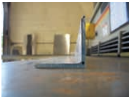
A stress analysis of this angle requires that the centroid of its cross-sectional area be located. (© Russell C. Hibbeler)
