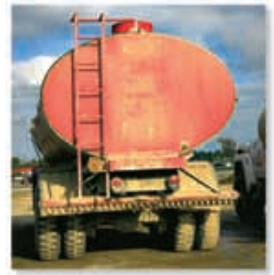
The resultant force of the water pressure and its location on the elliptical back plate of this tank truck must be determined by integration. (© Russell C. Hibbeler)
