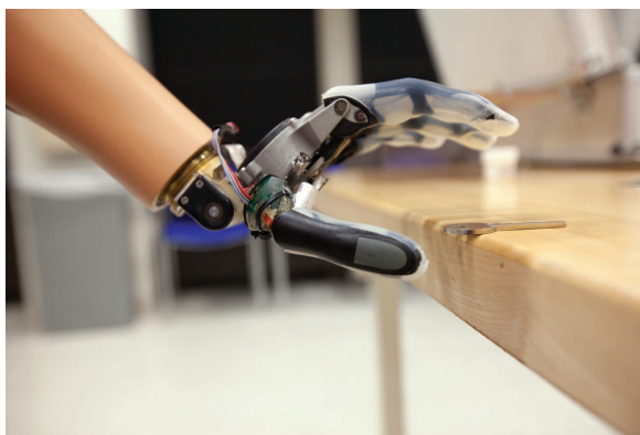
Photo 6.5 Frames and machines contain multi-force members. Frames are fully constrained structures, whereas machines like this prosthetic hand are movable and designed to transmit or modify forces.
