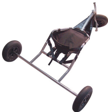
Photo 11.1 The center portion of the rear axle of the sport buggy is in pure bending.
