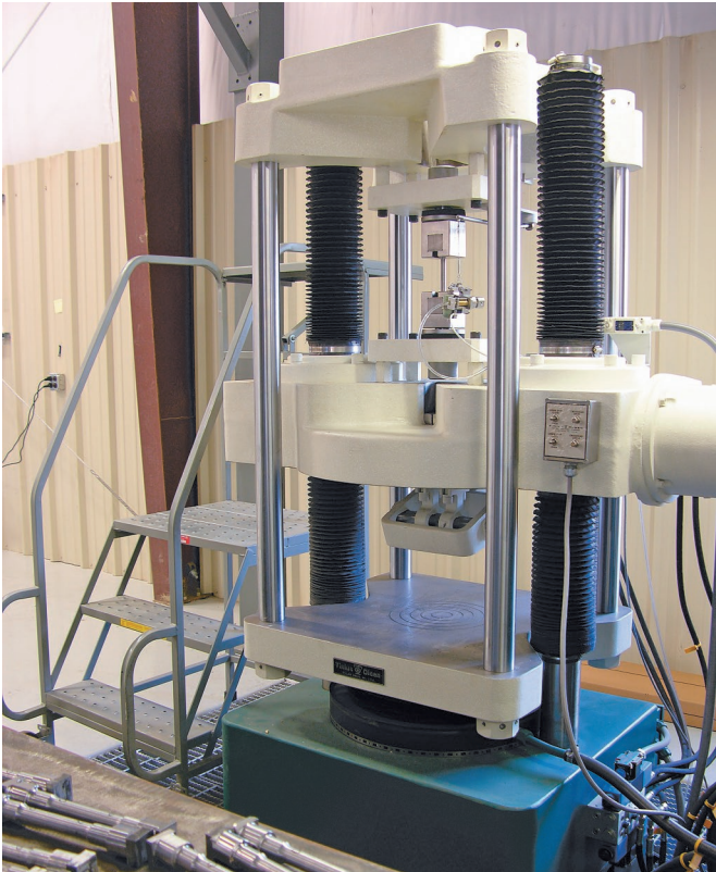
Photo 9.2 Universal test machine used to test tensile specimens.
