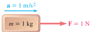
Fig. 1.2 A force of 1 newton applied to a body of mass 1 kg provides an acceleration of 1 m/s 2 .
