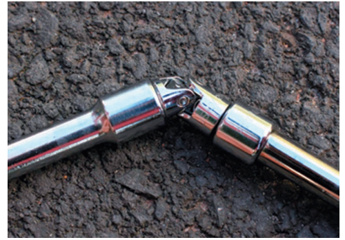
Photo 4.3 Universal joints, seen on the drive shafts of rear-wheel-drive cars and trucks, allow rotational motion to be transferred between two noncollinear shafts.
