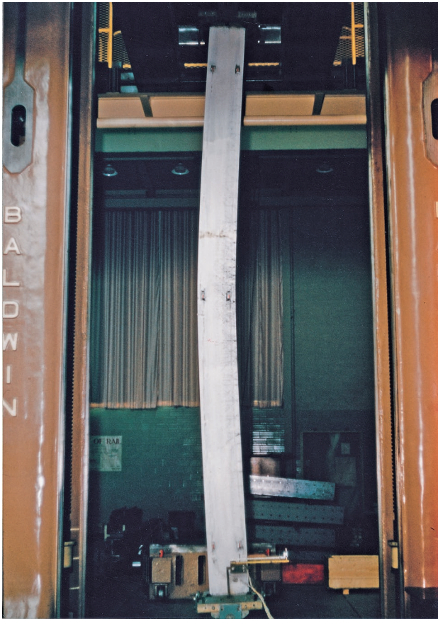
Photo 16.1 Laboratory test showing a buckled column. Courtesy of Fritz Engineering Laboratory, Lehigh University
