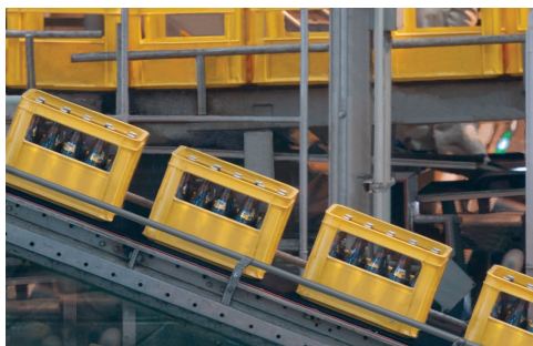
Photo 4.6 The coefficient of static friction between a crate and the inclined conveyor belt must be sufficiently large to enable the crate to be transported without slipping.
