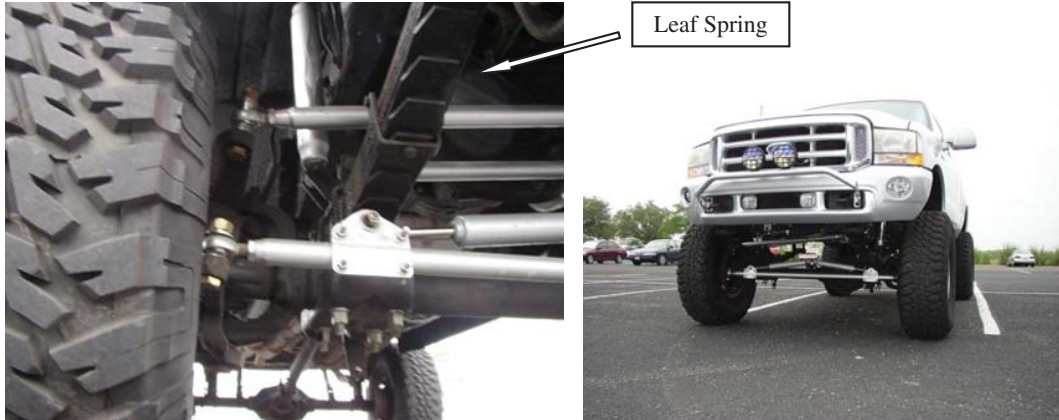
Figure 4.5.5 Vehicle suspension with translational springs and dampers
