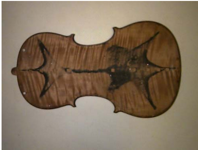
Figure 4.6.4 Distributed deflection response of a violin shaken at resonance. Reproduced with permission from Renaud Carpentier and Emmanuel Bossy, University of New South Wales
