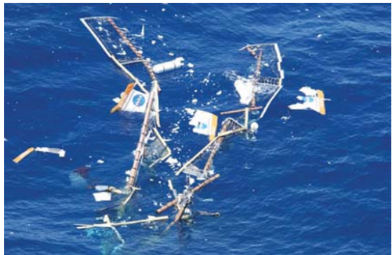
Figure 4.6.1 Prototype solar–electric aircraft shortly before and after failure due to vibration. Reproduced with permission from NASA
