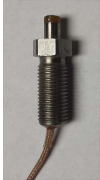
Figure 12.4.2 Noncontacting sensor to measure position of the spinning shaft
