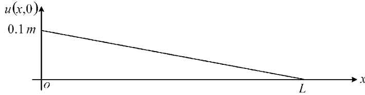
Figure E5.4.1(b) Initial deflection of the platform relative to its static equilibrium (Sag) state
