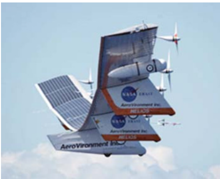
Figure 4.6.1 Prototype solar–electric aircraft shortly before and after failure due to vibration. Reproduced with permission from NASA
